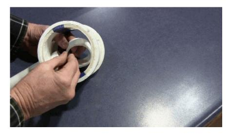
Page 4 of 35 Zip Tie Domes 1857 Brindley Hollow Road, Buffalo Valley, TN 38548 USA www.ziptiedomes.com - Telephone: (931) 858-6892 Tighten the Zip\_Tie to Secure the Center Ring to the Strut.
