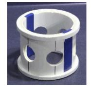
The Dual Covering Hubs have an extra ridge at the edge of the hub that allows you to attach the greenhouse plastic to the hub by cinching the zip ties over the plastic above the ridge, which secures the plastic to the hub.
