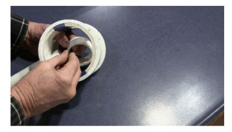
Tighten the Stainless Steel Zip Tie to Secure the Center Ring to the Strut.
