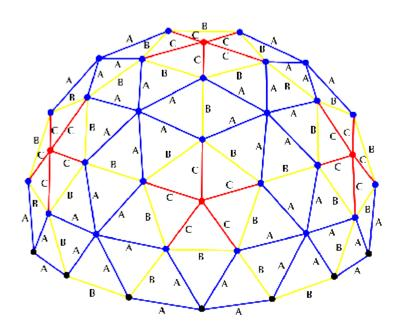
You may have to flex the hub up and down to get the struts to fit into the hub.
