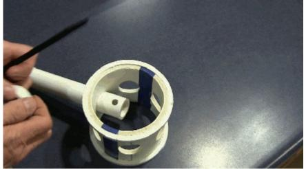
Insert a Stainless Steel Zip Tie into the end of the Strut.
